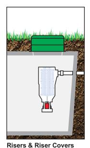
Polylok risers bring your septic tank cover to grade. This allows locating and servicing your filter easier and time saving by eliminating digging to find tank entrance.
